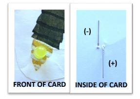
2. Take the LED and gently poke the legs through the cardstock in the center of the front of the card so the bulb is on the outside of the card and the legs are on the inside. Bend the short leg (-) upwards and flat against the paper and the long leg (+) downward and flat.
