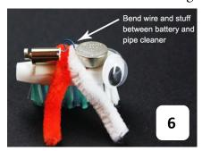
If the bristlebot does not turn on more pressure is needed in the connection between the battery and the wires. Try wrapping a rubber band around the battery to more firmly secure it in place.
